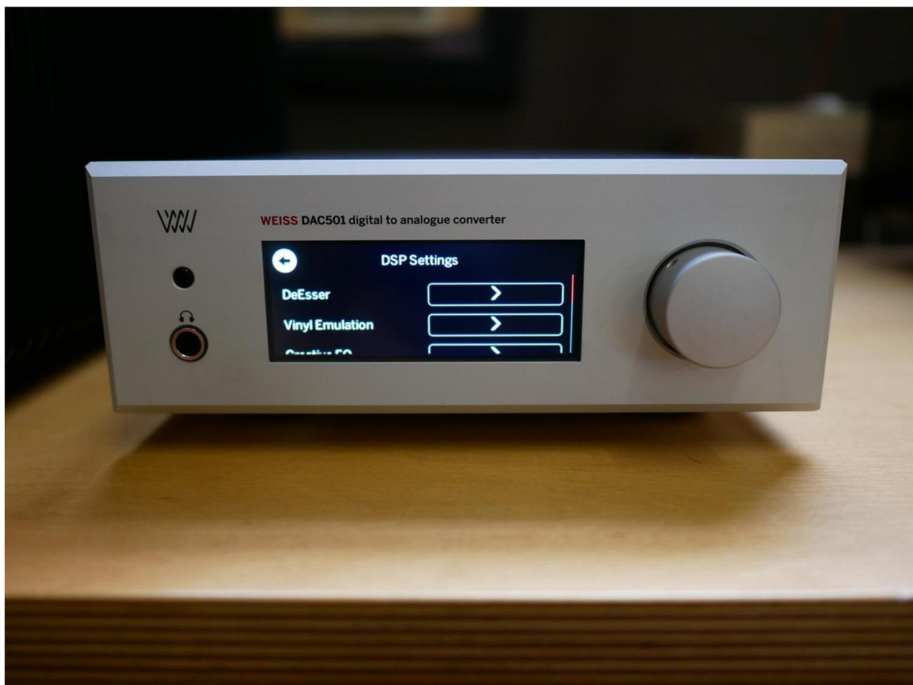
The DAC501’s front panel is deceptively simple with a color touch screen LCD display, 1/4” headphone jack, and a multi-function knob. Weiss includes a plastic remote that offers a number of useful functions, many are also available via the touchscreen as well, but the company recommends using the DAC’s web interface for those ready to dig into DSP. I happen to find the DAC501’s size, 18.8cm x 30cm x 7.2cm (W x D x H), a welcome change. The main difference
